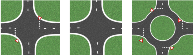
Figure 3: Available road topologies (RTAP), Straight Across Path (SAP)) and the direction from which the other vehicle is coming (Left Direction (LD), Opposite Direction (OD), Right Direction (RD)). In all cases the other vehicle has the priority. Therefore, there are six scenarios for the crossroad topology: three for Left Turn Across Path (LTAP/LD, LTAP/OD, LTAP/RD), two for Straight Across Path (SAP/LD, SAP/RD) and one for Right Turn Across Path (RTAP/LD). These scenarios are repeated with different setups where the starting position and the cruise speed for the dummy-vehicle change, so the interaction between the two vehicles always varies.
