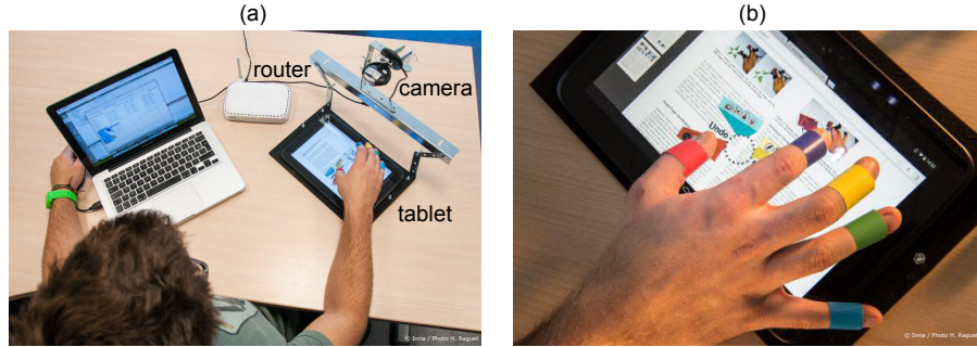
Figure 13: Finger identification technique used for the tablet and smartphone: (a) a camera is mounted on a frame fixed to the tablet or smartphone; (b) coloured rings are attached near each finger tip.
