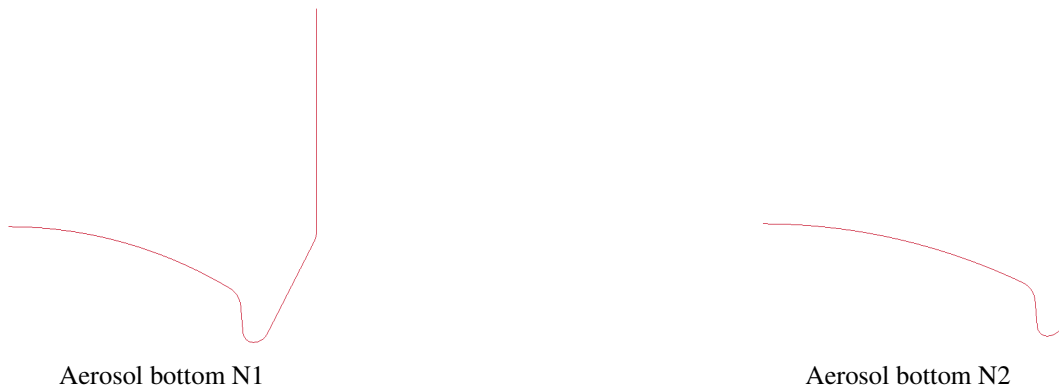
Figure 9. The two shapes of the aerosol can’s bottom used in our study ( N1 and N2 )
