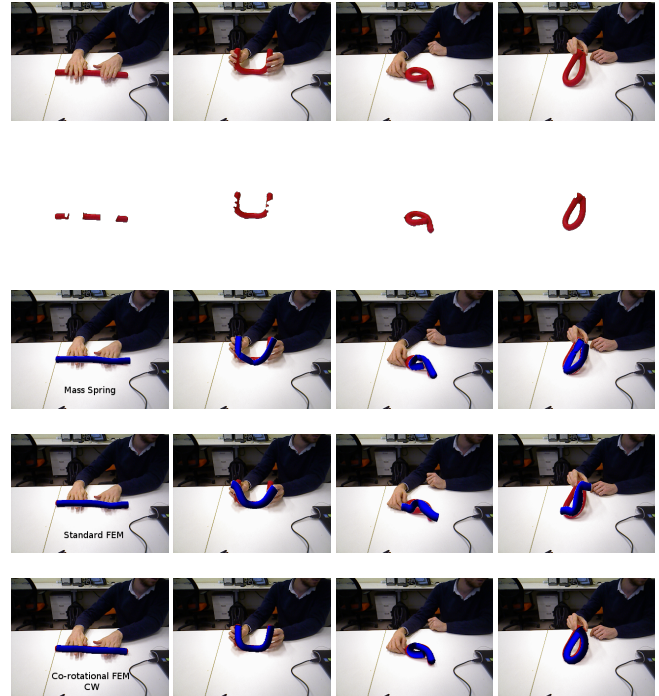
Fig. 9: Results of the tracking process for the cylindrical bar object, with the input images (first row), the segmented frames (second row), and the registered mesh reprojected in the input image, for the mass spring model (third row), the standard FEM model (fourth row) and finally with our approach.
