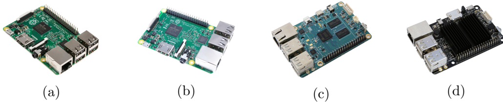
Figure 5: Single-Board Computers under test: (a) RPi2, (b) RPi3, (c) OC1+, (d) OC2.
