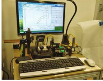
Fig. 6. Experimental test bench for contact/tripping force measurement.
