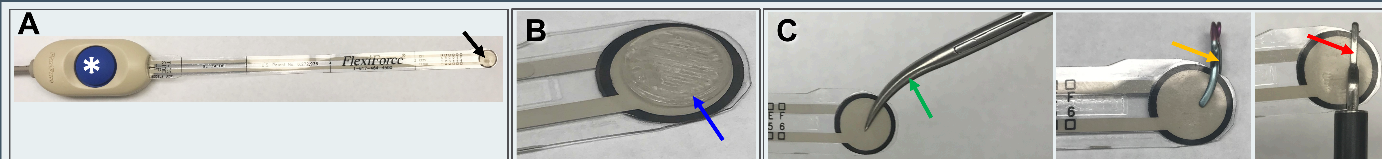
Figure 1 Calibration. Calibrating the force sensor, TekScan's Flexiforce ELF System, involved multiple steps. A: Preparing the sensor. After inserting the sensor (black arrow) into its adaptor (white asterisk), it first needed to be "broken in," which involved applying a force with one's finger that maxed out the default force settings 3-4 times. B: Weight calibration. First the force reading was zeroed. Next, based on the approximate force being tested, a predetermined maximum weight (ex. 1000 g) was applied to the sensor on top of a small 3D printed disk (blue arrow) that ensured the entire weight was detected by the force sensor, and the sensitivity setting was optimized. Then, each of the three predetermined weights (ex. 1000 g, 500 g, 200 g) were set on the printed disk 5 times. With those 15 data points, the Flexiforce ELF System computed a linear relationship to analyze the unknown crush forces. C: Crush force analysis set-up. Left to Right: Smooth, curved hemostat (green arrow), Aneurysm clip (yellow arrow), Crush tool (red arrow). Each method underwent 20 crush trials, and the average, standard deviation (StdDv), and 95% confidence interval (C.I.) were measured. The crush tool's dimensions required a non-centered force reading. To remain consistent, the crush force of the hemostat and aneurysm clip were analyzed over the same area of the sensor as the crush tool.
