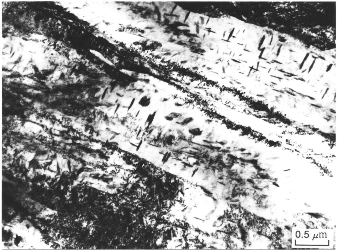
Fig. 4.10 TEM bright field image of lower bainite after 23 days of isothermal holding at 478 °C.
