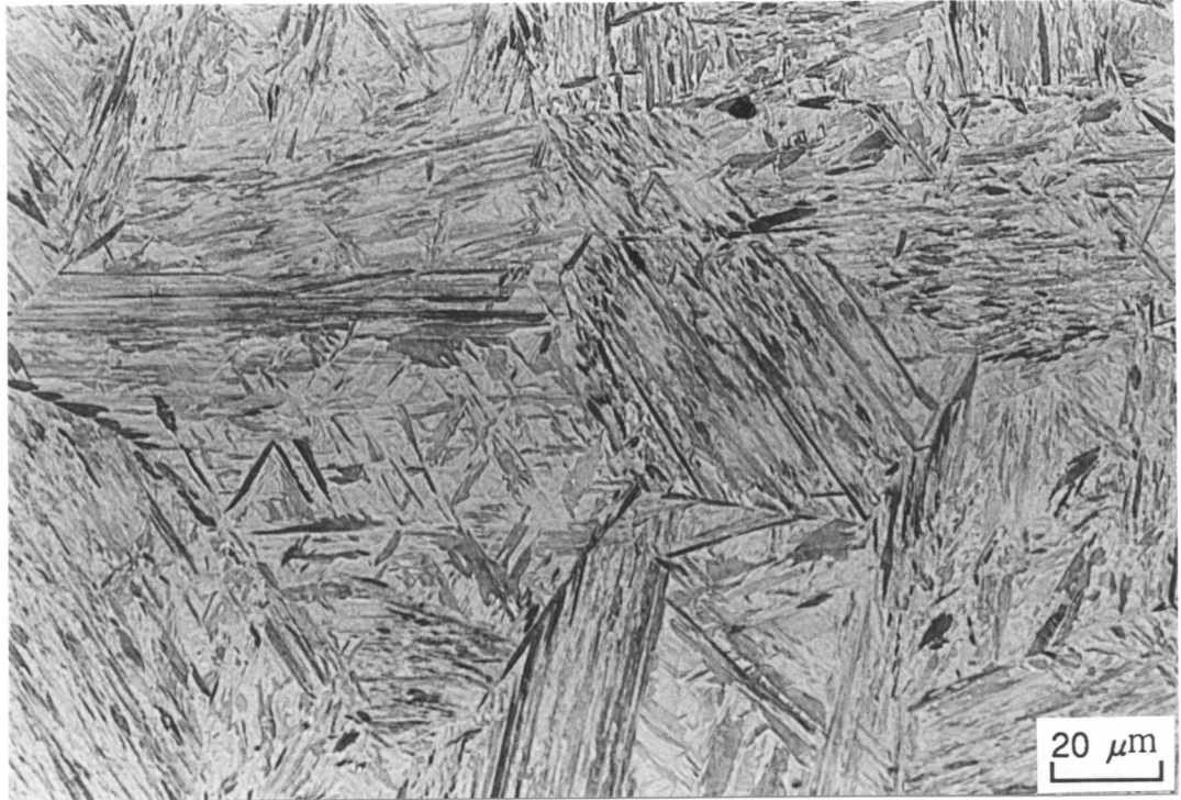
Fig. 6.1 Optical micrograph of martensite obtained by water quenching from 1100° C in the Fe-0.3C-4.08Cr wt.% alloy.
