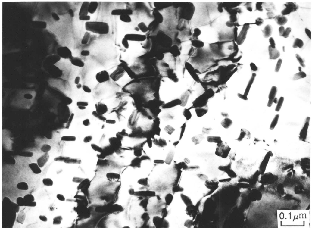
Fig. 6.9 TEM bright field image of a specimen helium quenched after 20 seconds of isothermal re-austenitisation from martensite at 790 °C in the Fe-0.3C-4.08Cr wt.% alloy.
