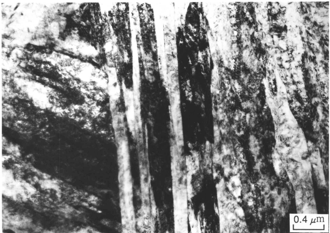
Fig. 6.2 TEM bright field image of martensite obtained by water quenching from 1100° C in the Fe-0.3C-4.08Cr wt.% alloy.
