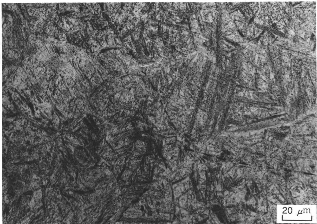
Fig. 6.31 Optical micrograph of a specimen water quenched after tempering of martensite at 700 °C for 51 hours.
