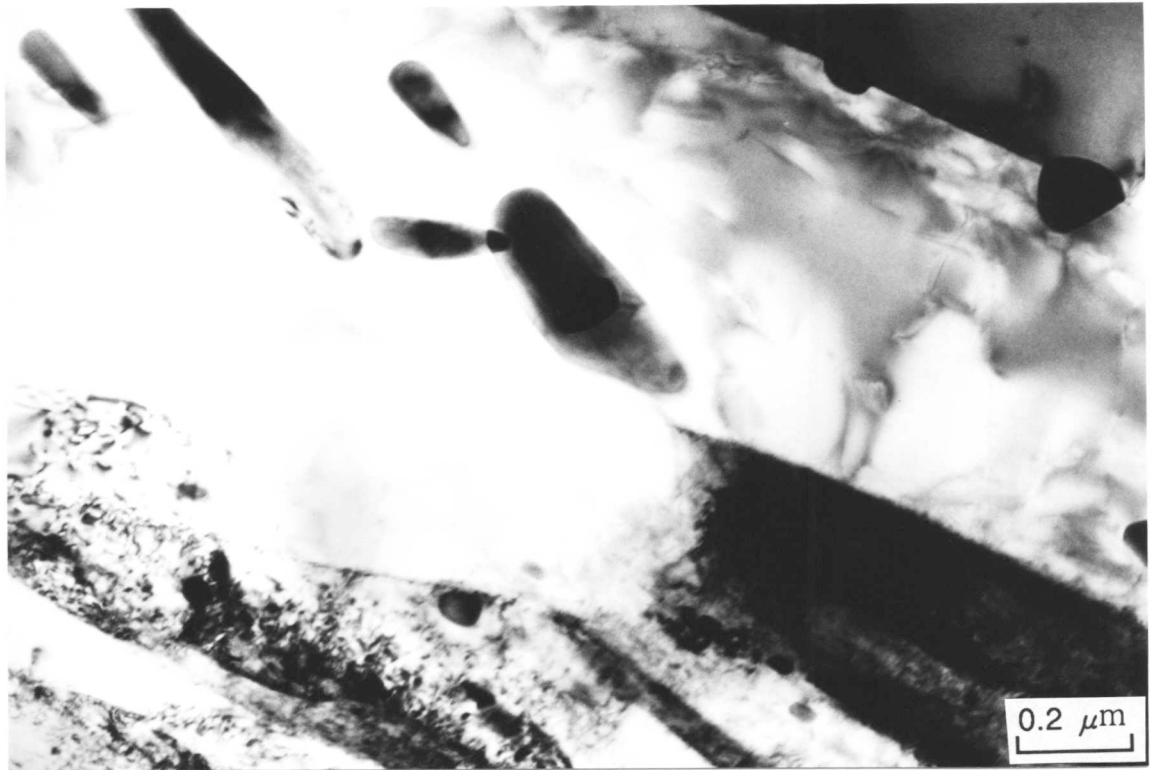
Fig. 4.18 TEM bright field image of a specimen re-austenitised at 778 °C.
