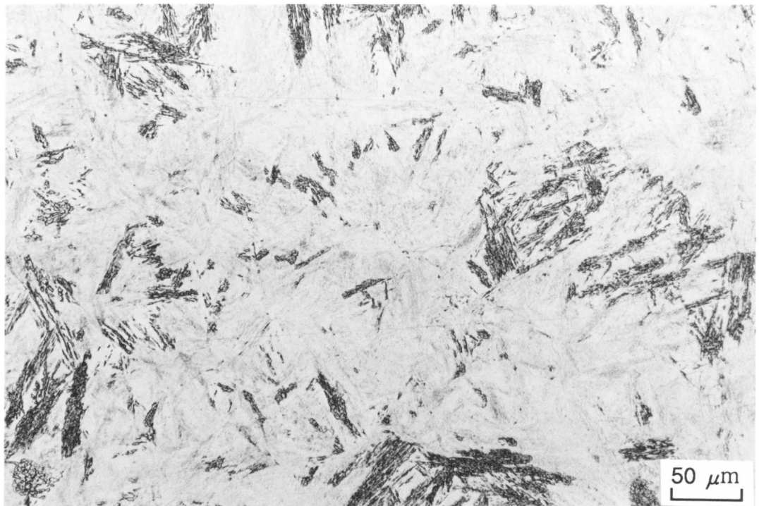
Fig. 4.15 Optical micrographs of isothermally reaustenitised specimens at a) 778 °C, b) 785 °C, c) 790 °C and d) 805 °C.
