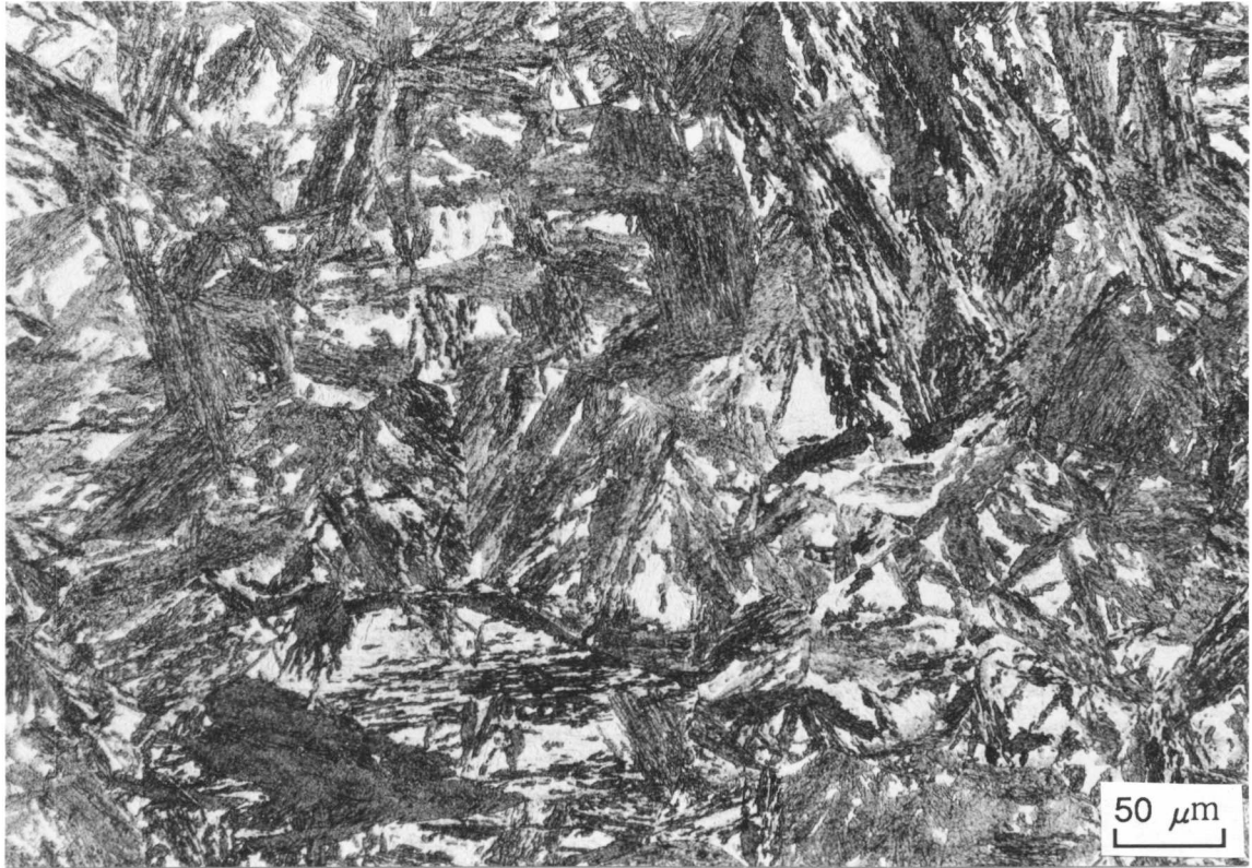
Fig. 4.8 Optical microstructure of a specimen helium quenched from 420 °C after bainite transformation.
