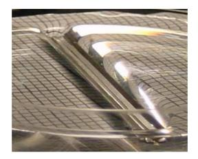
Figure 3.5: Photograph of a four-strip raft floating on water. Here the strips are made of stainless steel shim and are around 7 cm long and 2 mm wide.
