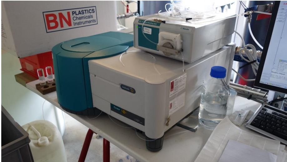
Figure 2.12: Field spectrophotometer (Vary Eclipse) with flow-through cell and peristaltic pump. The spectrophotometer was connected to a computer that continuously measured the tracer emissivities of water diverted from the pumping well.
