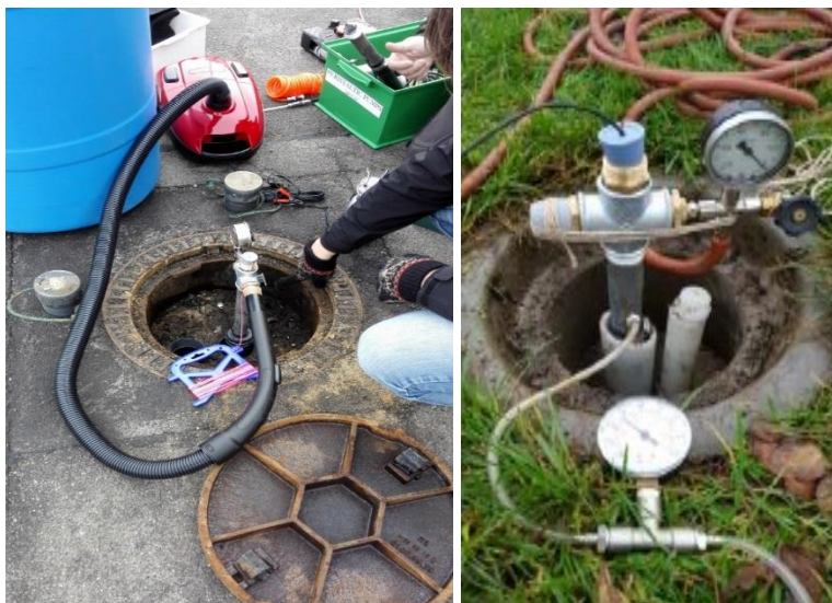
Figure 2.4: Slug test using a conventional vacuum cleaner (left). Slug test device installed in a borehole (right).
