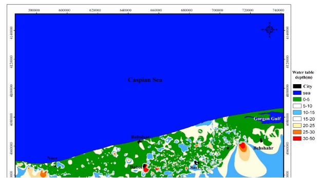
Figure 5. The map of average water table depth in the study area (m).
