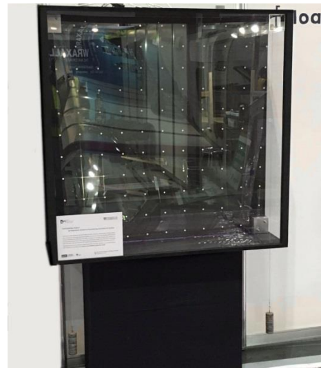
Fig. F1: Interactive set-up of cold bending thin chemically toughened glass by mechanical means.
