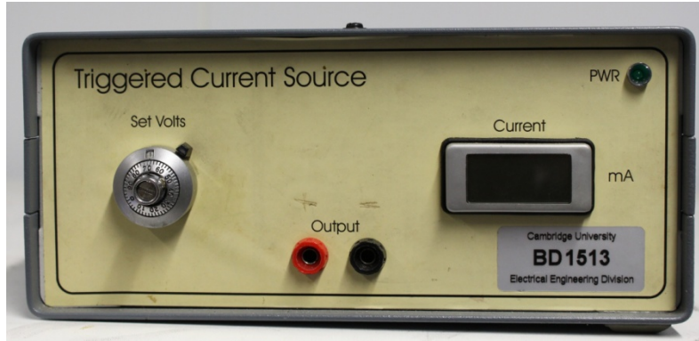
FIG. 3.9. Picture of the constant current source for the Hall sensor.
