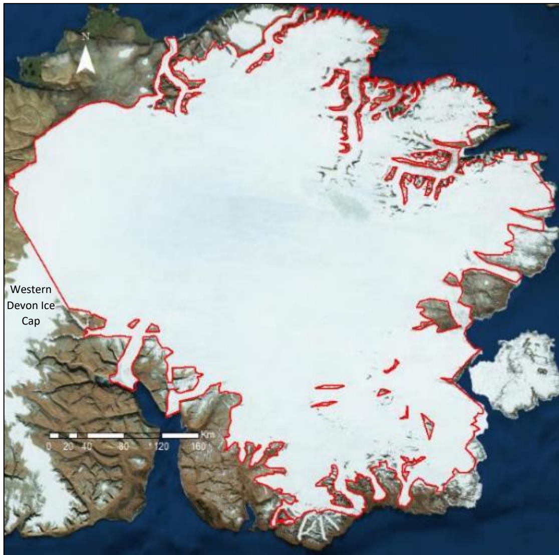
Figure 4.2. Red outline of the ice cap used for mesh generation and for clipping other datasets, superimposed on Landsat 7 imagery from summer 1999 (ArcGIS online, 2017). Nunataks too small to be accounted for in the mesh can be seen, and some areas not of interest, such as Western Devon Ice Cap, have been excluded.
