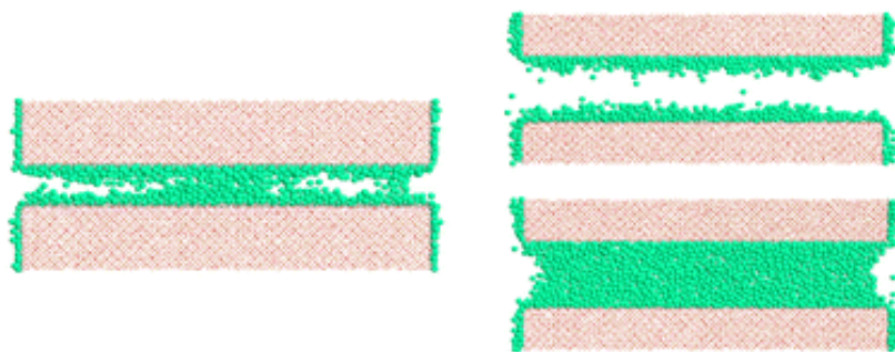
Fig. 1.4 Characteristic molecular configurations obtained using grand-canonical MC simulations for nitrogen adsorption in a MCM-41 pore with D = 24 \text{ \AA} (left panel) and D = 48 \text{ \AA} (right panel) [31]. The right panel shows two distinct fluid configurations at different pressure, before (upper panel) and after the adsorption (lower panel).
