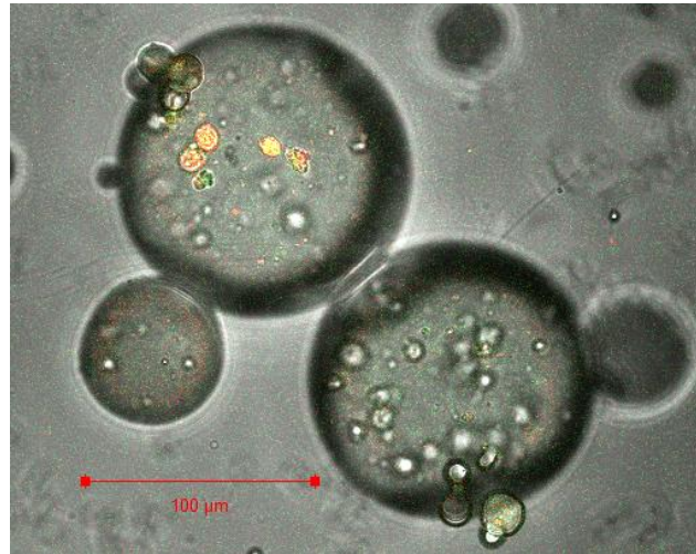
Figure 4.12: Confocal microscopy image of calcium alginate gel microbeads containing jurkat cells. These microbeads are spherical and mono-dispersed produced by using the optimised microfluidic setup and chip.
