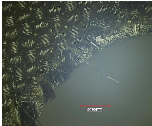
Figure 1.1 Fibre delamination of CFRP at the hole-exit in a mechanically drilled hole
