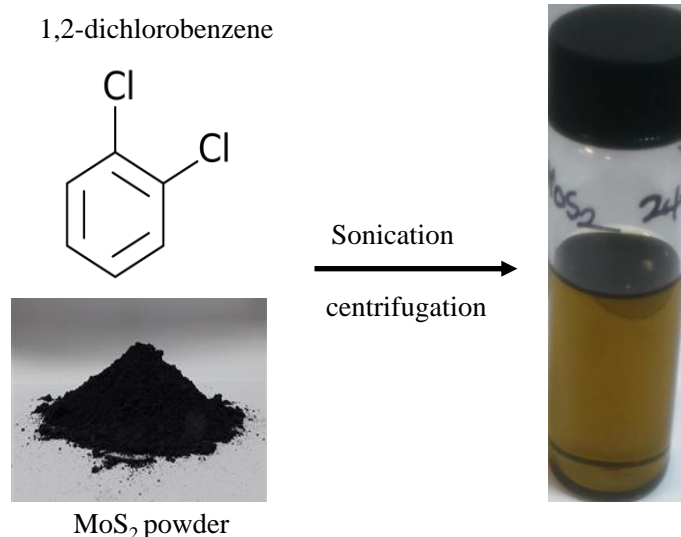
Figure 6. 1. Photographs of MoS 2 illustrating the different dispersion processing stages.
