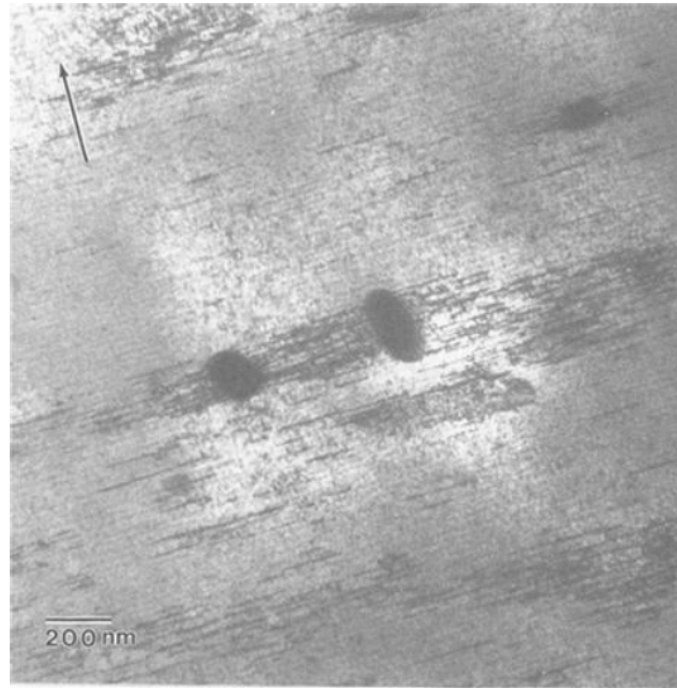
Figure 2-17 SPPs nucleating in the vicinity of Fe-Cr SPPs in Zy-4 after neutron-irradiation at 312 °C to 10 dpa in a PWR \sim 6 \times 10^{25} n m -2 .
