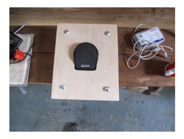
Figure 3: PD4 Buttons with tactile and haptic feedback
