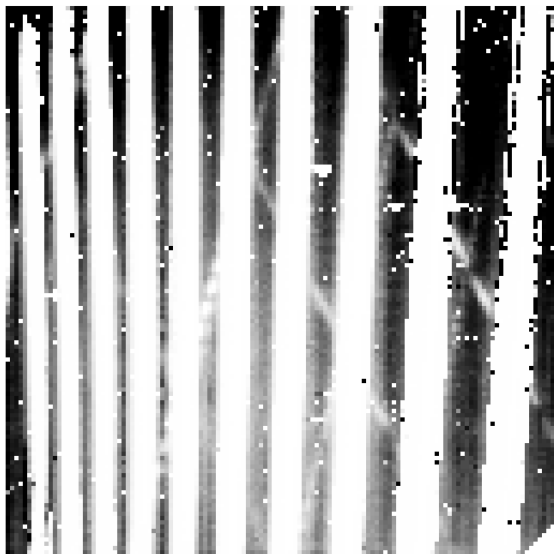
Fig. 1.— LH detector image ( 128 \times 128 \text{ px}^2 ) of a heavily saturated source. Vertical white bands show the 10 individual spectral orders in which the source is observed. For each spectral order, the wavelength axis is approximately vertical and the cross-dispersion axis is approximately horizontal. In the text we refer to rows and columns to describe the detector rows and columns in a given spectral order. The detector shows in this case artifacts in the form of several diagonal streaks. This artifact is different from the background gradient presented in Fig. 2.
