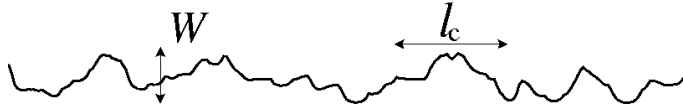
Fig. 5.1 Example of a rough interface characterized by a lateral correlation length \ell_c and the global width W(L, t) .
