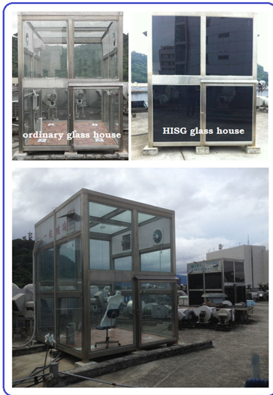
Figure 4. Photograph of the test houses constructed for outdoor testing.
