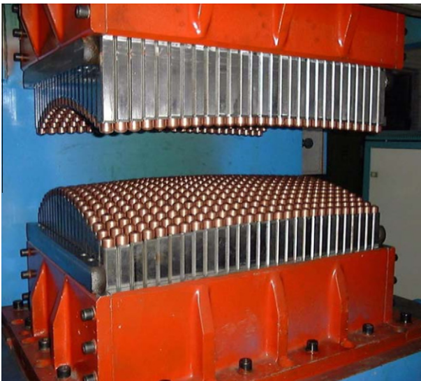
Fig. 1. Reconfigurable mould for sheet metal processing [1].
