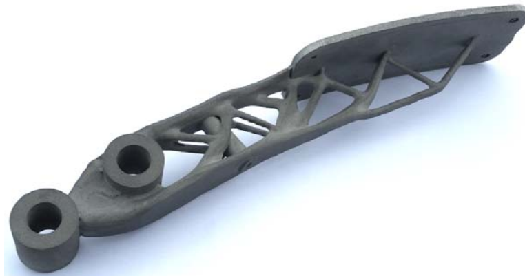
Figure 11 Manufactured topology optimised brake pedal with lattice designed foot pad (see online version for colours)
