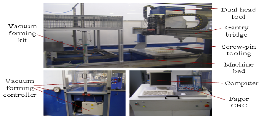
Fig.5 The completed HAVES
