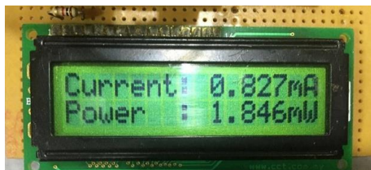
Figure 3.43: LCD Screen Displays the Load Current and Power Consumption
