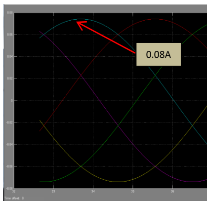
Figure 4.13: Current (A) from 5-phase PMSG 3 m/s wind speed (Peak 0.08A)
