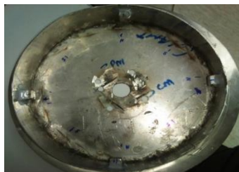
Figure 3.24 (a): Magnet poles glued with epoxy on stainless steel casting
