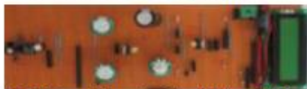
Fig. 5.4: Energy Harvesting Circuit Built on Stripboard
