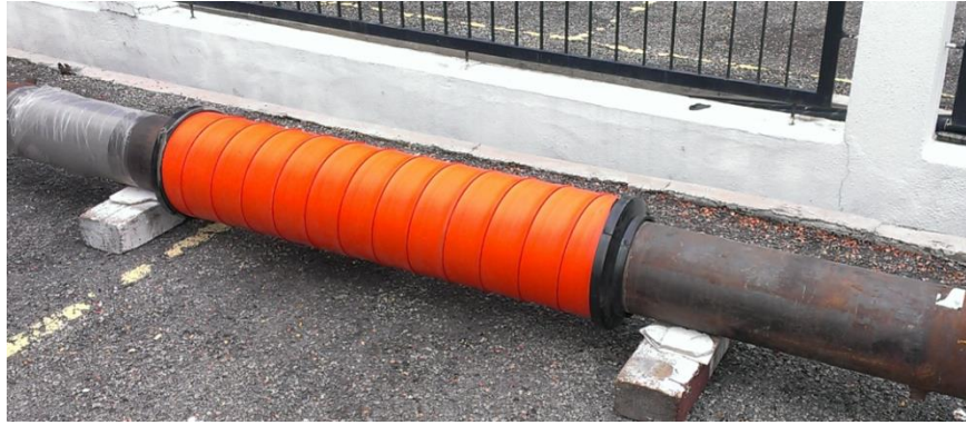
Figure 4-21, API 5L grade X52 steel pipe with Helicoid Epoxy Sleeve™ system installed
