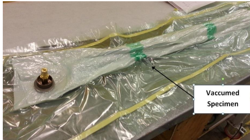
Figure 5-10, Curing of the composite prepreg performed with the aid of vacuum bagging
