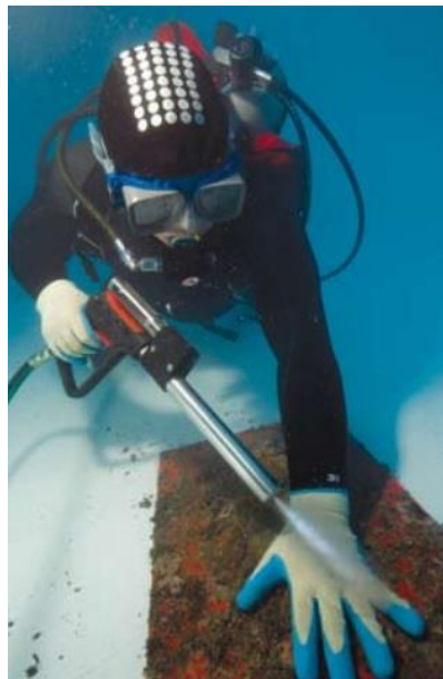
Figure A-8, Diver operating the Cavidyne CaviBlaster™ (CaviDyne, 2014)
