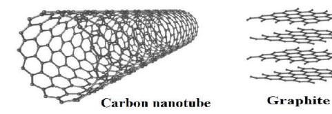
Figure 3. Some examples of carbon allotropes. (Original sketches by Michael Strock)
