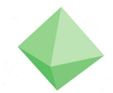
Figure 2. An Octahedron. Each of the 8 faces is of equal proportions. Both, the tetrahedron and the octahedron are Platonic solids.
