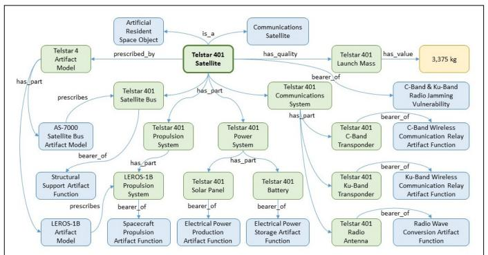
Fig. 2. A partial representation of components of the Telstar 401 satellite along with their design specifications and functions. Blue nodes represent classes in the Space Object Ontology. Green nodes represent instances of an SOO class. Yellow nodes represent values of an instance. Labeled links represent relations that hold between the linked nodes.
