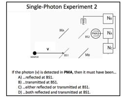
**FIGURE 1.** This sample concept question can serve to generate in-class discussion on the differences between experimental data and a physical interpretation of that data. [BS = Beam Splitter; M = Mirror; PM = Photomultiplier; N = Counter.]
