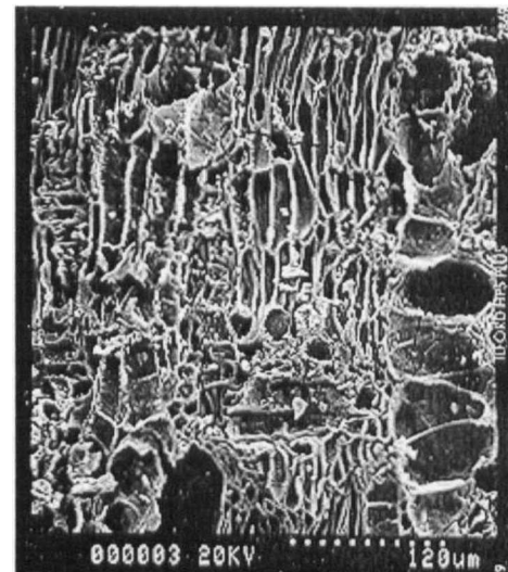
Plate 18 Fraxinus (left column: transverse section, right column-top: transverse, middle-bottom: radial)
