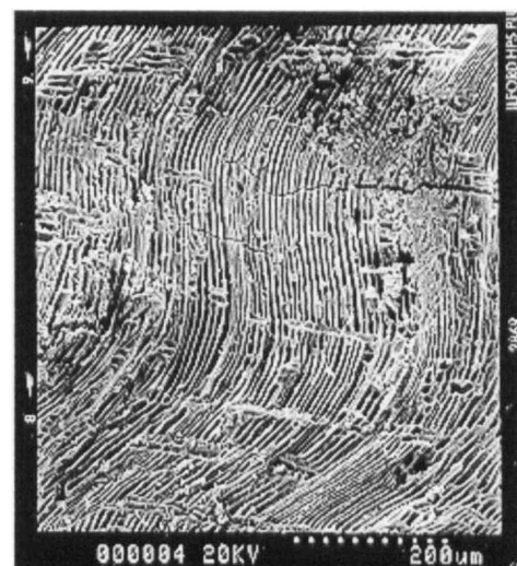
Plate 38 Thermal degradation and possible signs of wood deformation other than fungal decay; top & middle: twig ( Ulmaceae ) showing fissures in rays, bottom: Juniperus fragments showing signs of compression (left) and wavy patterns (right)
