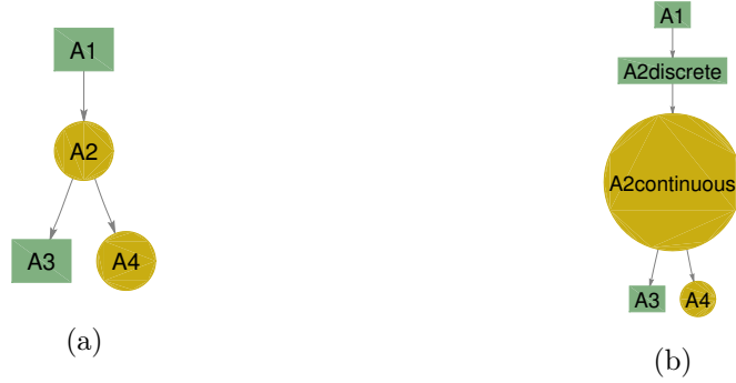
Figure 8: Graphical representation of the discretization procedure: on the left hand side the initial structure, on the right hand side the structure resulting from the discretization of the node A_2
