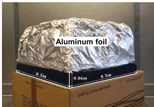
Fig. 8 The RF absorber with its pyramids covered by aluminum foil. The size of its base is marked.
