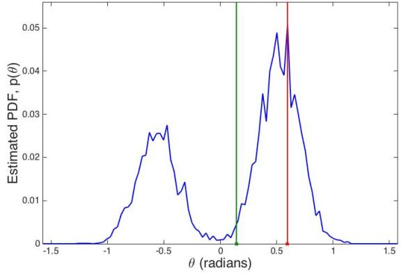
Fig. 5. Example multi-model estimated probability density function for helicopter pose angle ( $\theta$ ) for filter C (nonlinear drag model). Average (estimated) value for pose angle shown in green, and the actual pose angle in red.
