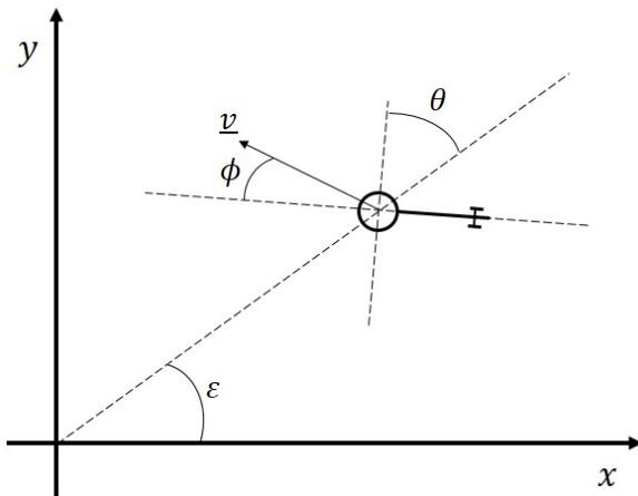
Fig. 1. Geometry showing sensor axes, helicopter orientation and velocity vector.
