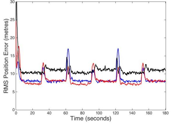
Fig. 4. RMS position errors for manoeuvring helicopter scenario shown in Fig. 3. Black curve is filter A (baseline Kalman). Blue curve is filter B (constant drag model). Red curve is filter C (nonlinear drag model).
