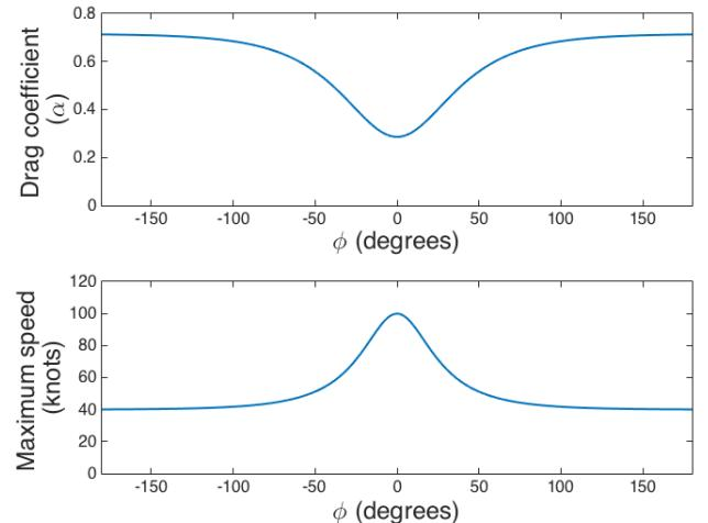
Fig. 2. Example of nonlinear drag function and maximum speed as functions of the angle  $\phi$  between the longitudinal body axis and the velocity vector.
