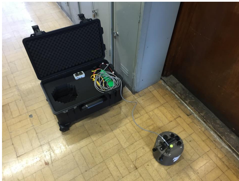
Figure 4. Force-Balance Accelerometer on Site
