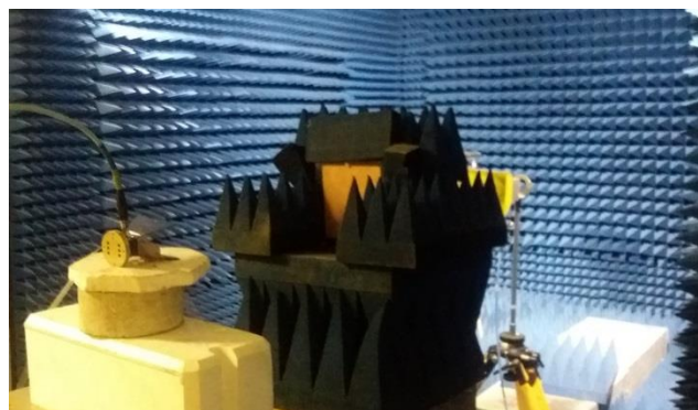
Fig. 15. Measurement setup to measure the transmission coefficient of the FSS.
