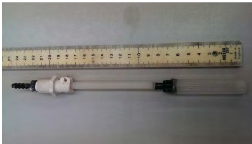
Figure 4-3: Laboratory float valve designed for tubular electrode use.
