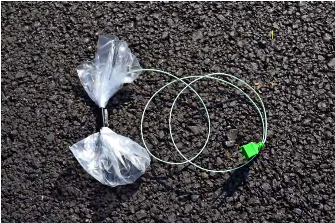
Figure 5-12: K-Type thermocouple in protective bag ready for insertion.
