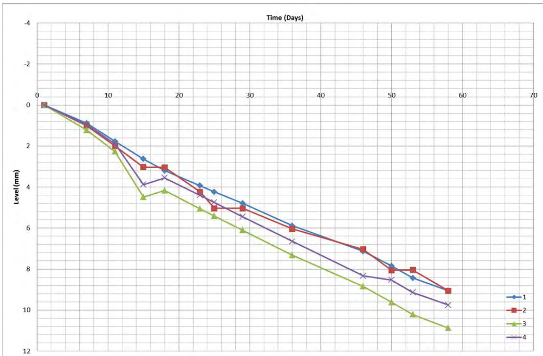
Figure 7-18: Site trial control footing levels.
