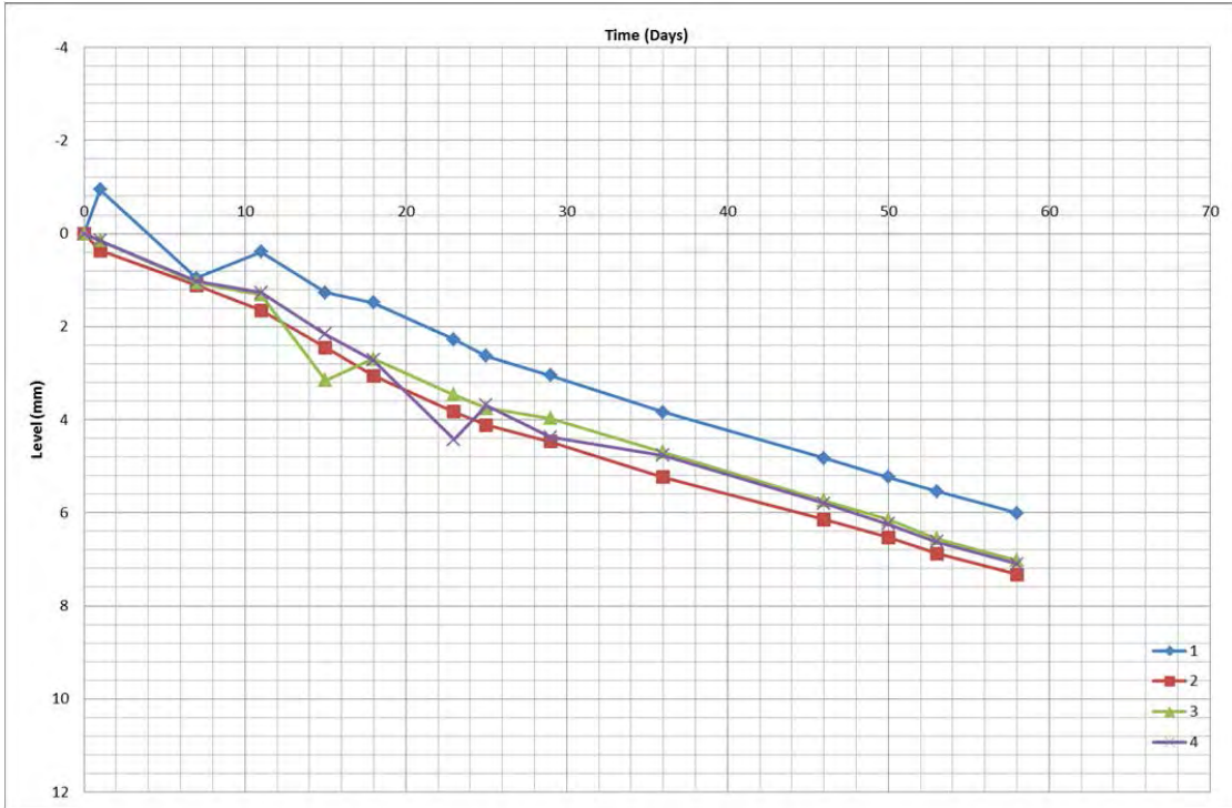
Figure 7-17: Site trial vertical electrode trial footing levels.
