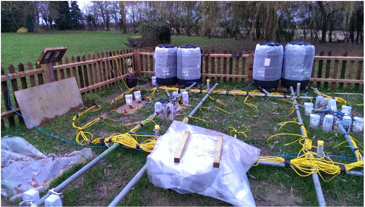
Figure G-20: Completed setup with resistivity array
