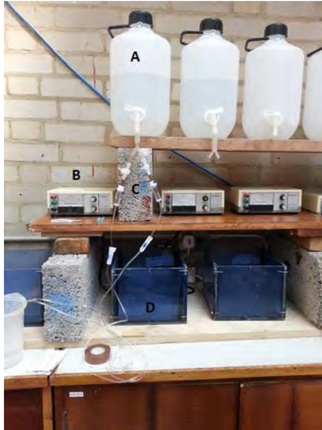
Figure 4-10: Current intermittence trial setup. A: Fluid containers, B: Power supplies, C: Flow regulators and D: Electrokinetic test cells.
