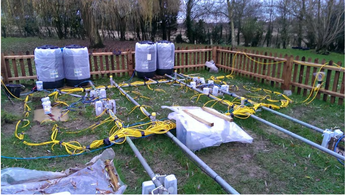
Figure G-19: Completed setup with resistivity array
