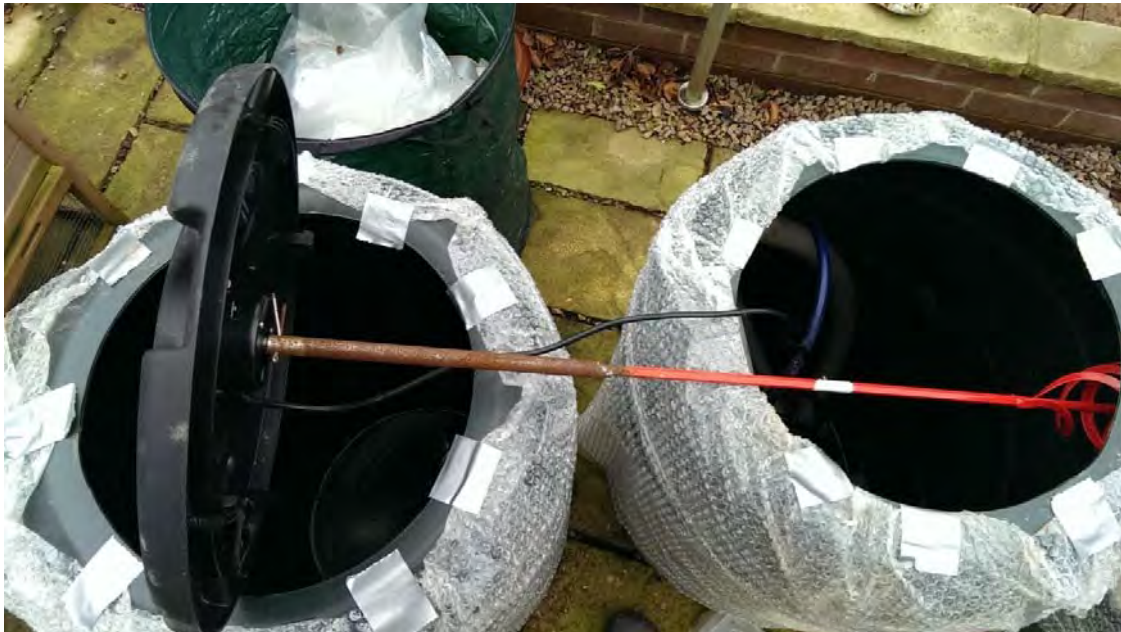
Figure 5-17: Water butt stirring mechanism attached to the base of the water butt lid.
