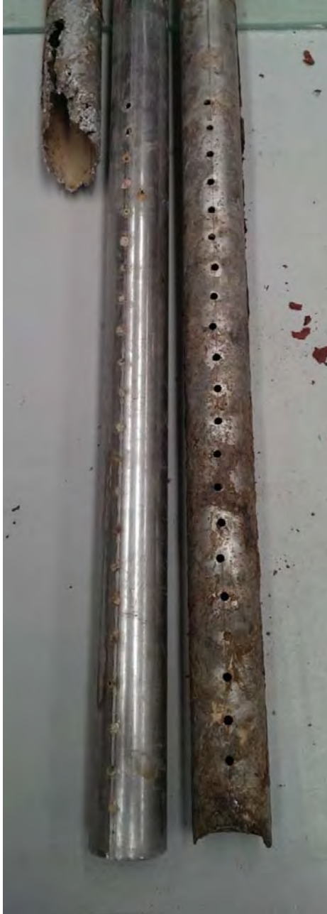
Figure 7-38: Raked electrodes after use. Anode – Cathode – Anode (1A1 – 1C – 1A2).
