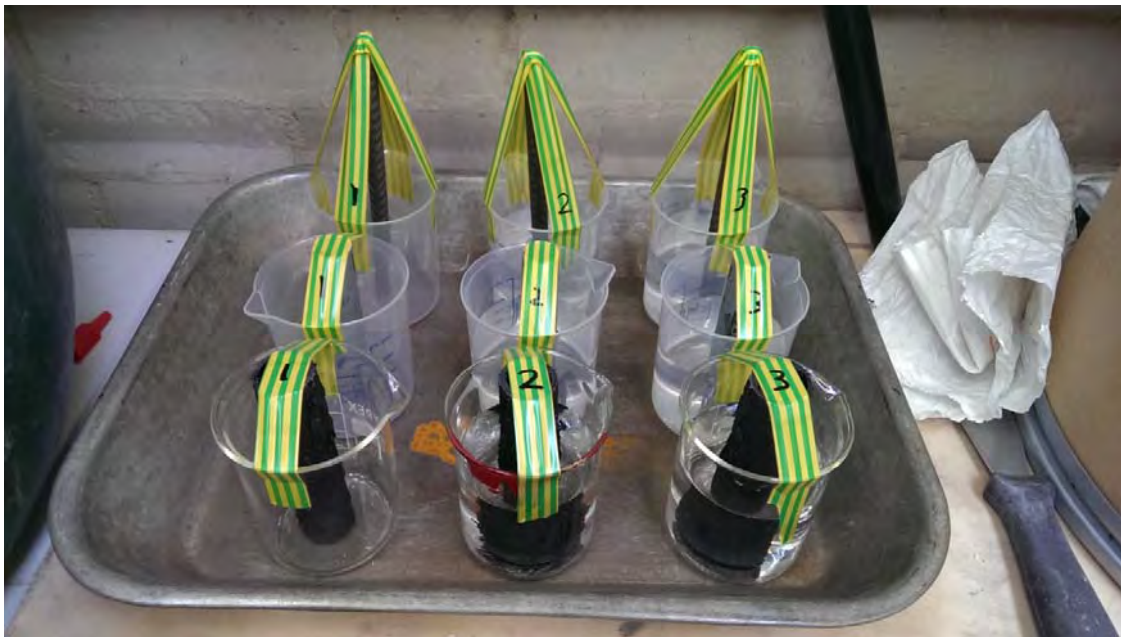
Figure 4-7: Electrode decay test setup before sealing inside box.
