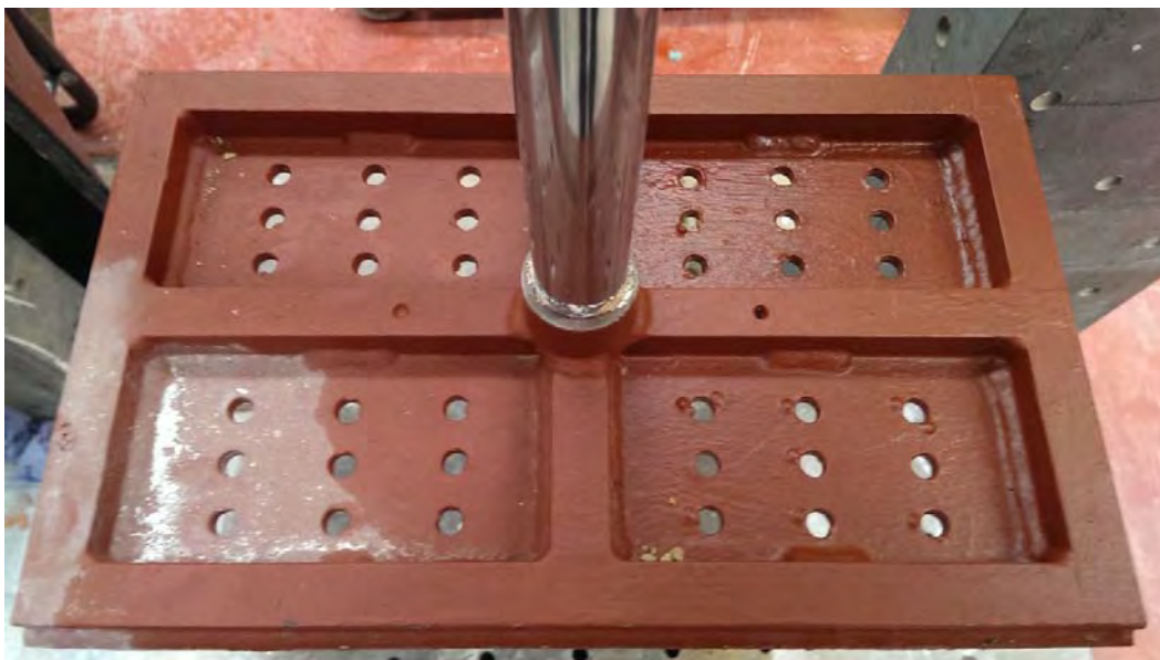
Figure 4-5: Consolidation load plate.
