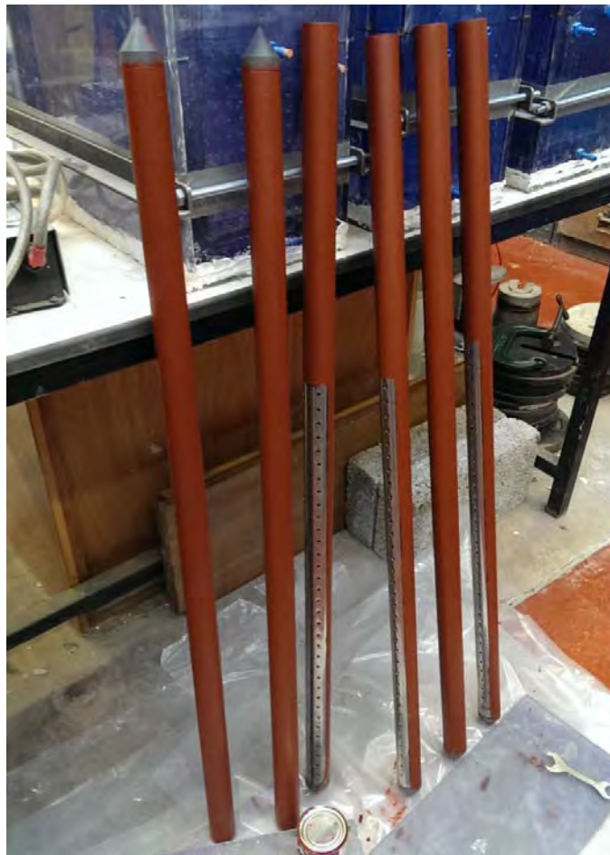
Figure 5-16: Site trial electrodes with end caps and red oxide paint cover.
