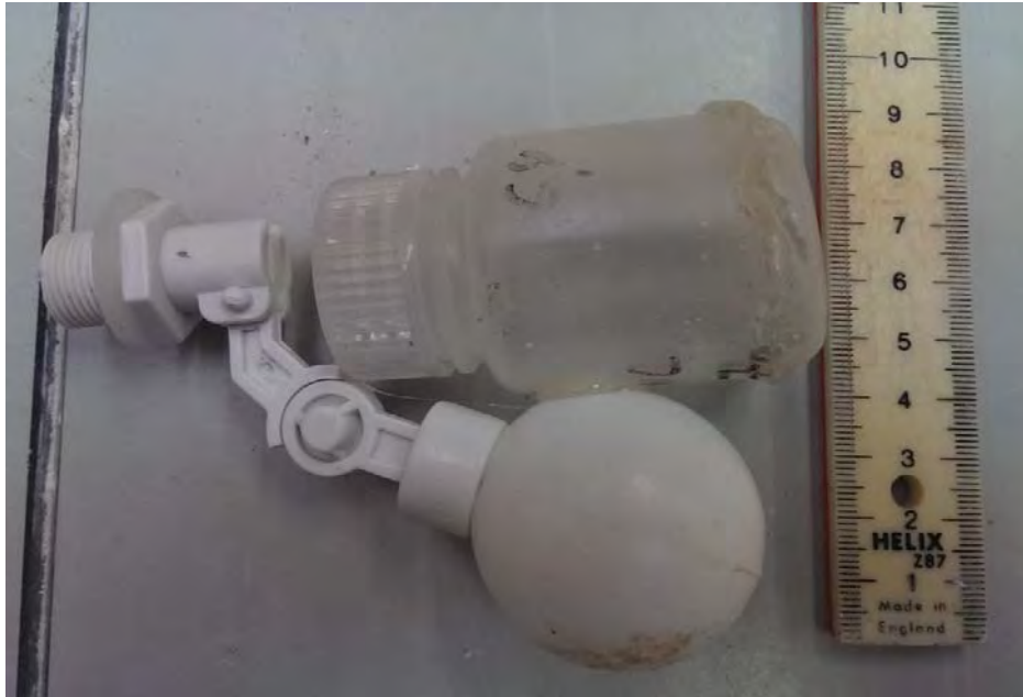
Figure 5-15: Modified float valve from within the electrode topper.
