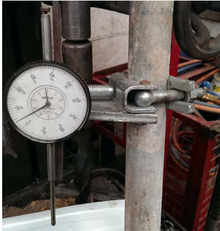
Figure 5-10: Dial gauge with fabricated scaffold mount.
