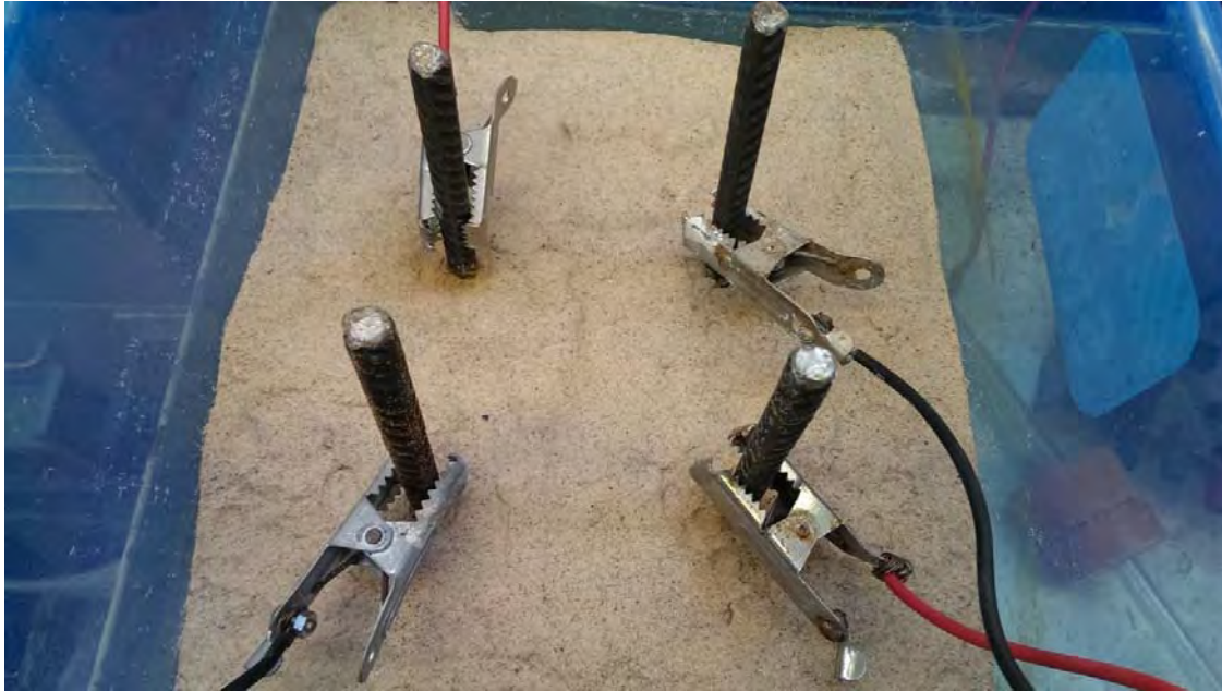
Figure 4-9: Electrode polarisation of a four electrode array in wet sand.
