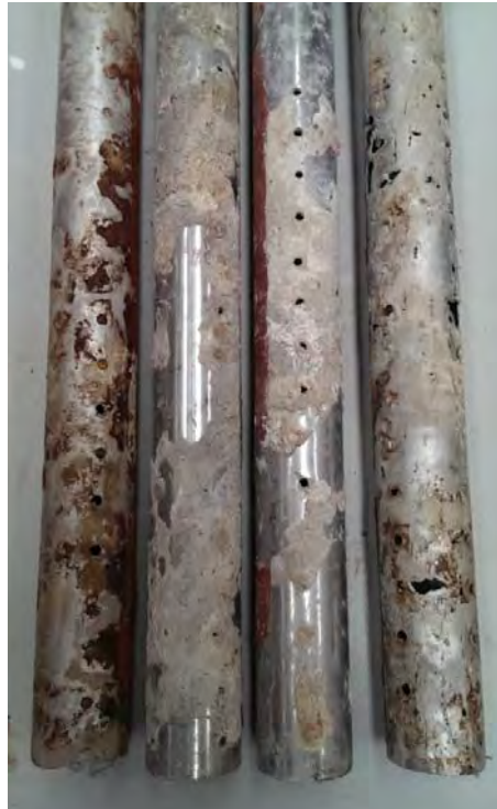
Figure 7-39: Vertical electrodes after use. Anode - Cathode - Cathode – Anode (21, 22, 23, 24).
