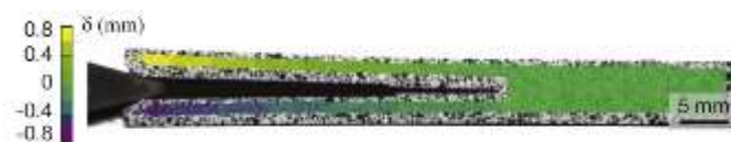
Figure 51 – Digital Image Correlation of speckle patterned double cantilever beam [159].
