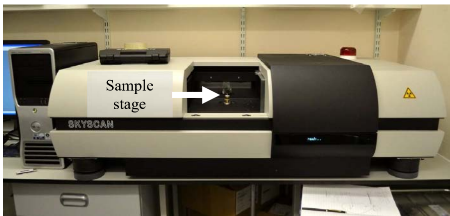
Figure 72 – SkyScan 1172 Bench-top X-ray micro-tomography system with sample chamber open. X-ray generation is through a 100keV Hamamatsu tube-source X-ray and the detector is an 11MPix CCD camera coupled to the device X-ray scintillator.
