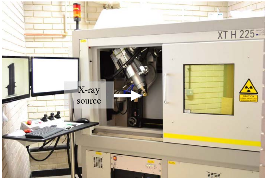
Figure 71 – Nikon XTH-225 industrial X-ray tomography system with sample chamber open.
