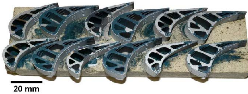
Figure 61 – Firebrick shelf used to load multiple aerofoil sections into furnace for high-throughput testing, showing a selection of alternating pairs of Pt (larger) and Pt-aluminide (smaller) aerofoil sections following three 20-hour cycles at 1200°C.
