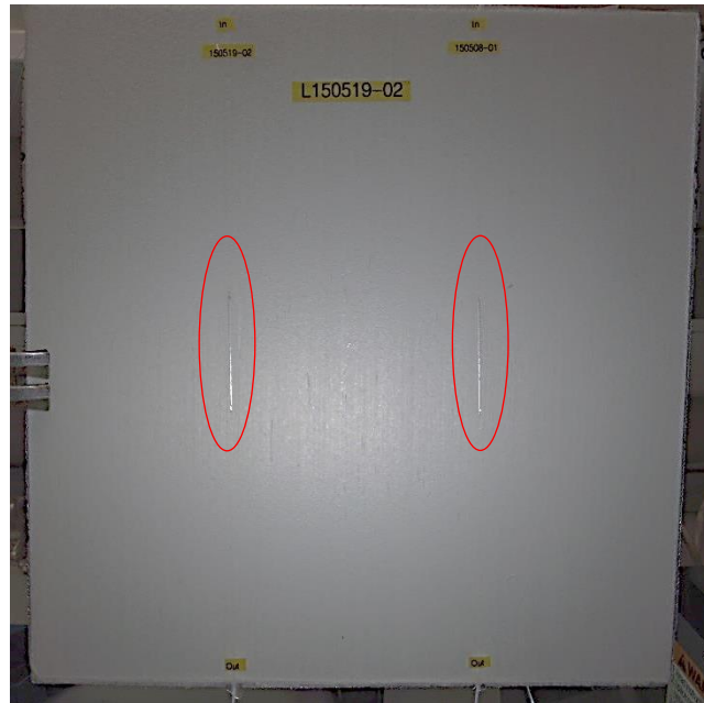
Figure 69 Detail of the two FOAES embedded into the laminate L150519-02 (red ellipses).
