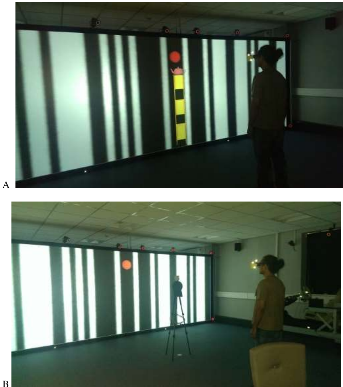
Figure 4. Study set up. Picture A shows a participant fixating on the background whilst a virtual foreground is present (-2m condition). Picture B shows a participant fixating on the background whilst a real foreground object is present (0m condition).
