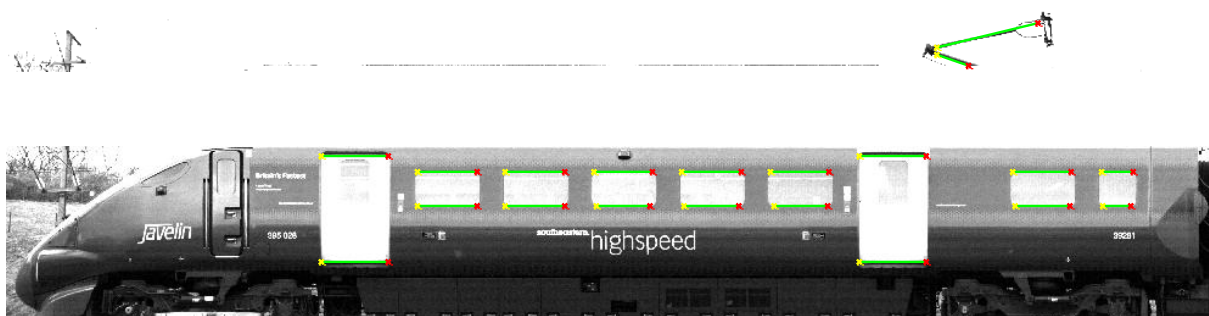
Figure 7.12- Hough Line transform processed image: (Top) Overhead line area, (Bottom) vehicle main body side view
