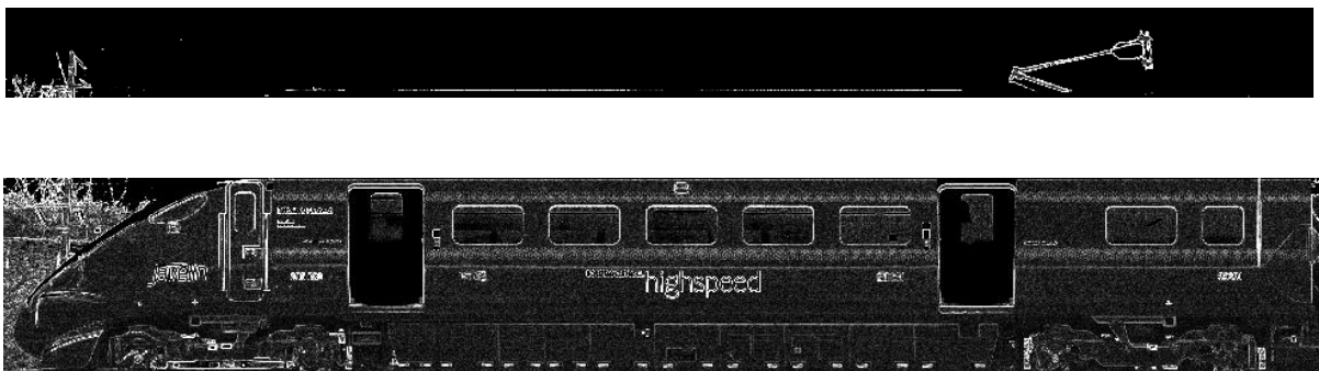
Figure 7.9- The image represented in gradient magnitude: (Top) Overhead line area, (Bottom) vehicle main body side view
