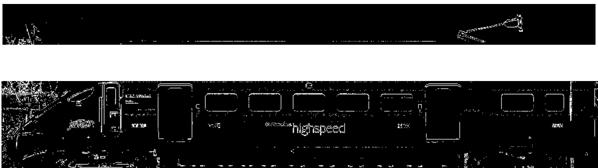
Figure 7.10- Edge detection processed image: (Top) Overhead line area, (Bottom) vehicle main body side view
