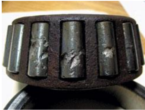
Figure 2.5- roller damage of tapered-roller-bearing [47]
