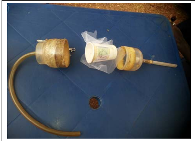
A: A colluzi and Petrarca type mouth aspirator for HLC with its different parts including in the middle a cardboard paper soup cup whose basis is replaced by a net in order not to block the air flow produced by the collector sucking.
