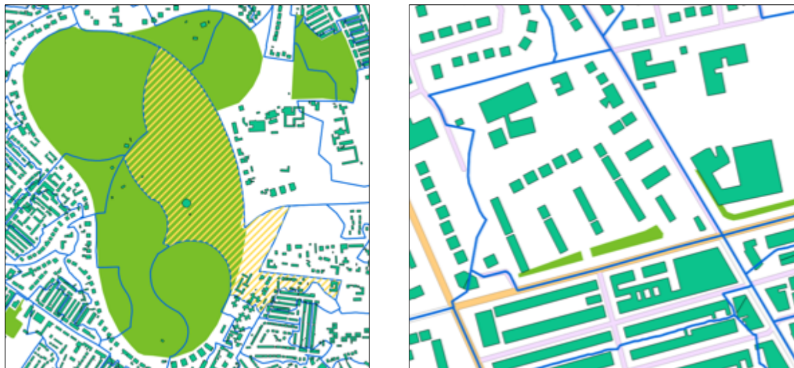
Figure 5.1 Maps looking at the un-generalised Output Area borders (blue lines). Left: Sefton Park, Liverpool. Notice how the area of the park is divided arbitrarily between proximal OAs (yellow hashed line pattern). Right: Output Area borders usually coincide with the street network, making simple street network-to-area assignments impracticable.
