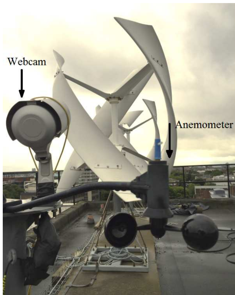
Figure 6.8: Anemometer and webcam on the roof for wind speed measurement and wind turbine monitoring
