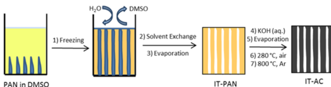
Figure 4.1. Schematic representation of the process employed to prepare the IT-ACs
