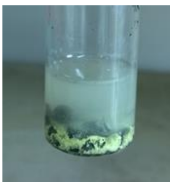
Figure 5.12. CPSS150 monoliths after addition of 2M HCl. A white/yellow precipitate forms immediately on addition of the acid with accompanied effervescence and \text{H}_2\text{S} odour
