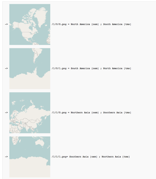
Figure 7.19: Describing how the globe can be represented by tiles. Source: OpenStreetMap Wiki (OpenStreetMap Contributors, 2014a)
