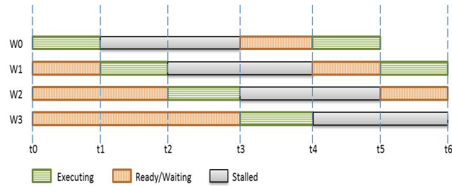
FIGURE 5.4: The GPU is able to hide latency by swapping out wavefronts/warps that stall during memory operations.
