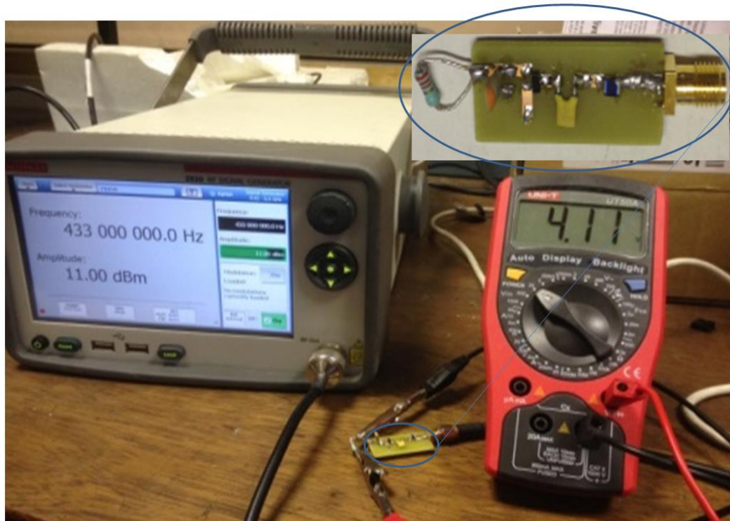
Fig. 3.8. The measurement setup of the rectifier circuit test experiment with a sweep of power input at 433 MHz.
