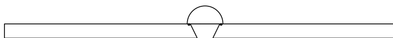
Figure 6.19: To-scale schematic representation of an alternative design to the existing top plate of the flow cell. The area of contact between the two liquids is limited to a disk of 9-mm diameter. The flow cell is sealed by a 10-mm hemisphere pushed onto an O-ring.
