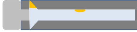
Figure 4.1: Schematic representation of the quartz cuvette with an oil drop in the aqueous phase. Not to scale.
